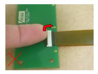
• The actuator opens by rotating it in the direction OPPOSITE to the direction of the insertion of the FPC. DO NOT attempt to open it from the same side as the insertion of the FPC.
